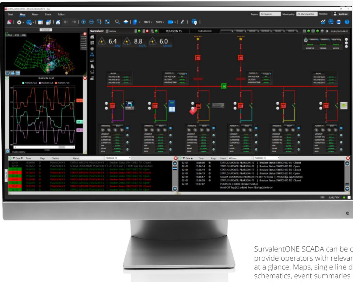
SurvalentONE SCADA can be configured to provide operators with relevant information at a glance. Maps, single line diagrams, schematics, event summaries & alarms are shown in the SmartVU application.
