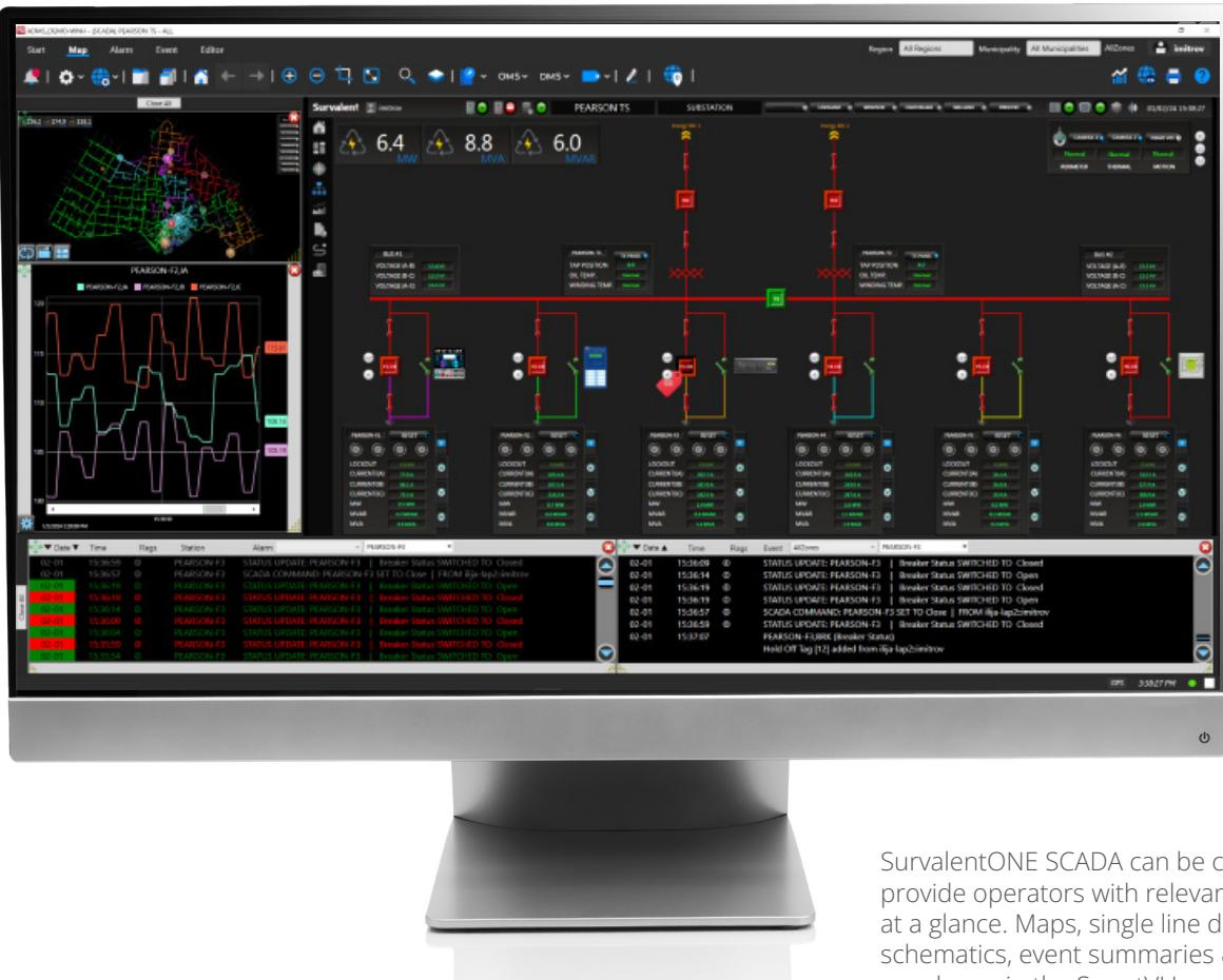
SurvalentONE SCADA can be configured to provide operators with relevant information at a glance. Maps, single line diagrams, schematics, event summaries & alarms are shown in the SmartVU application.
